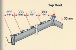
How to instal lisplank (MULTI ROOF)
